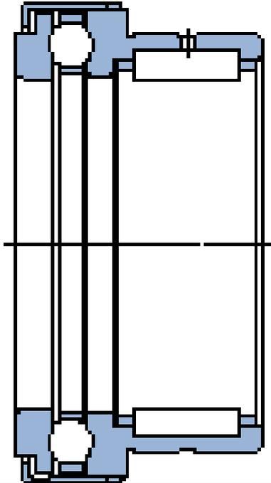
**NKX 40 Z SKF Nadel-Axial-Rillenkugellager NKX..Z**
