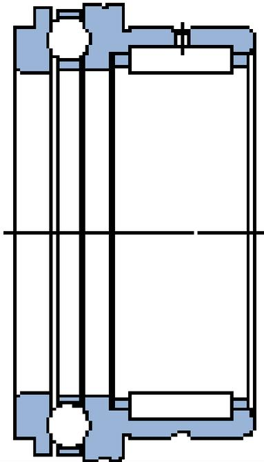
**NKX 45 SKF Nadel-Axial-Rillenkugellager NKX..**
